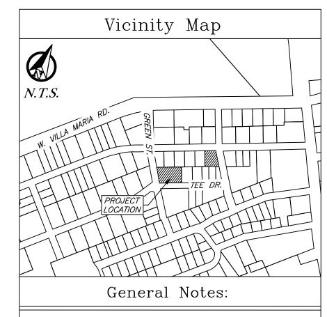
Bearing system shown hereon is based on the Texas Coordinate System of 1983, central zone (4203), grid North as established from GPS observation using the Leica Smartnet NAD83 (NA2011) EPOCH 2010 multi-year CORS Solution 2 (MYCS2).
